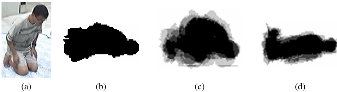
Fig. 5.2 An example of error type 2. (a) An ambiguous posture. (b) The normalized silhouette of (a). (c) The average normalized silhouette of squatting 45°. (d) The average normalized silhouette of kneeling 45°.
