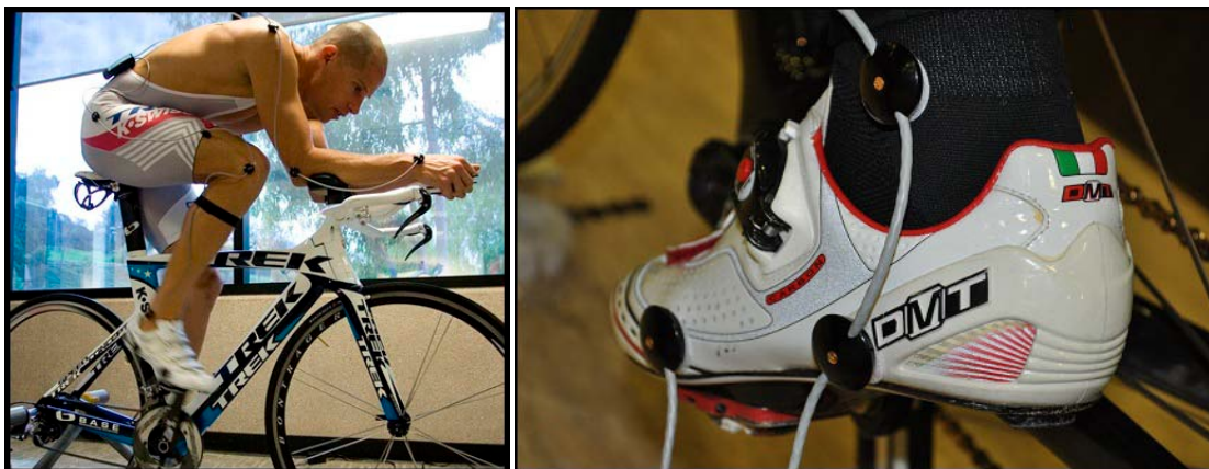
圖 13 RETUL LED harness(左)；圖 14 RETUL 追蹤運動員腳踝姿勢(右) (RETUL, Inc., 2007)
