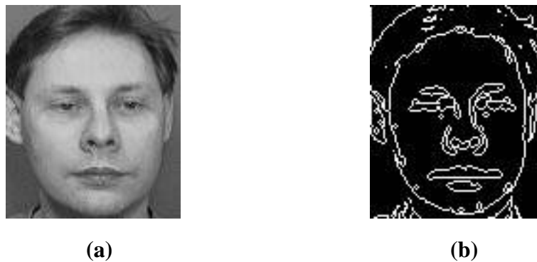
Fig. 2.1.2 (a) Original face image (b) Face image after applying Laplacian edge detector.
