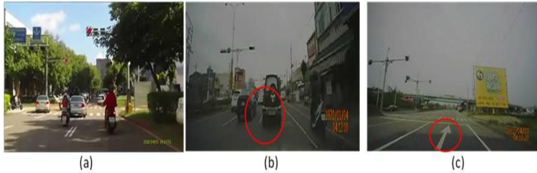
Figure 1-3 : Different driving environments. (a) The presence of shadows. (b) The lane line occluded by the vehicles. (c) Various markings on the road.
