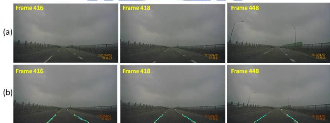
Figure 4-8 : The straight lane line case. (a) Original images. (b) Output images.
