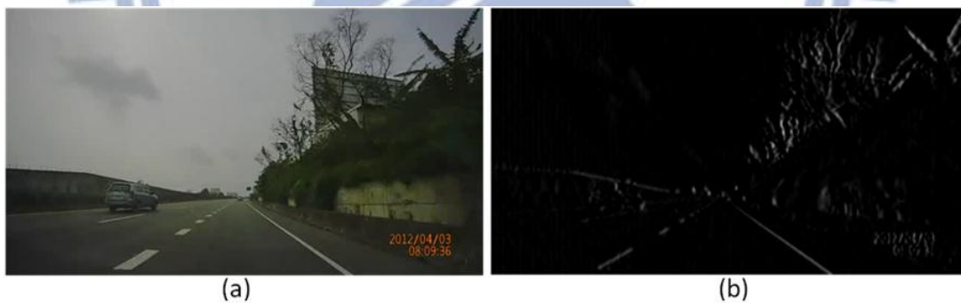
Figure 3-5 : An example of edge detection result. (a) Original image. (b) Result of edge pixels which have positive responses after using G_x .
