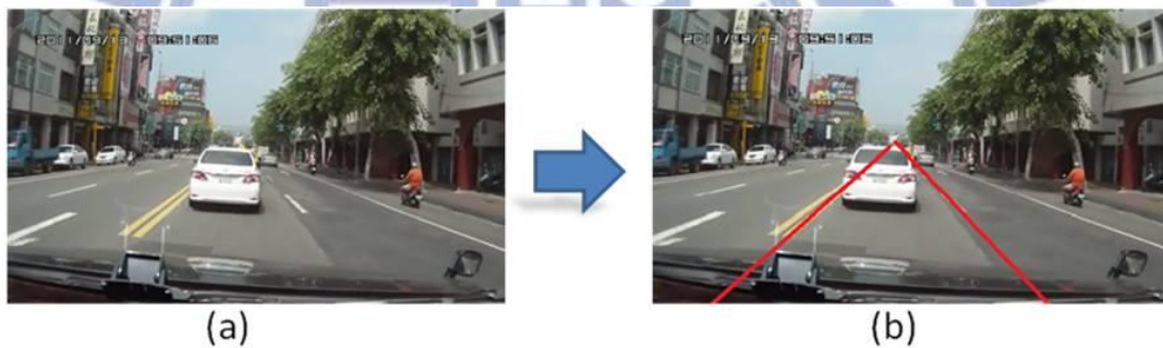
Figure 1-1 : An example of the lane line detection. (a) Input frame captured from the camera. (b) Output frame where the position of the lane lines is located.
