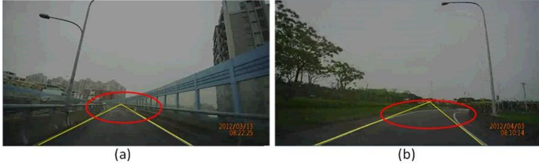
Figure 3-9 : The unreasonable representation of the curve lane lines. (a)(b) The curve lane lines in the red circle cannot be detected, and only the straight lane lines in the near field are detected.
