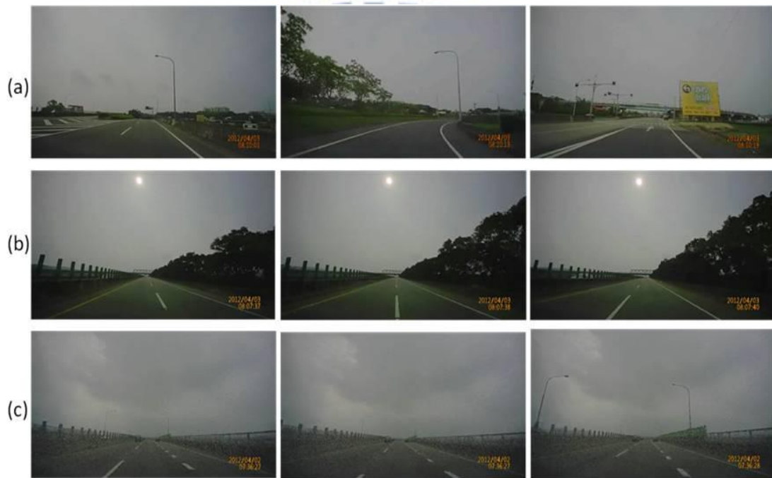
Figure 4-1 : Sample road images in different cases. (a) Intermediate case where the type of lane lines is from the straight to the curve then back to straight. (b) Lane changing case from left to right. (c) Straight lane lines case.
