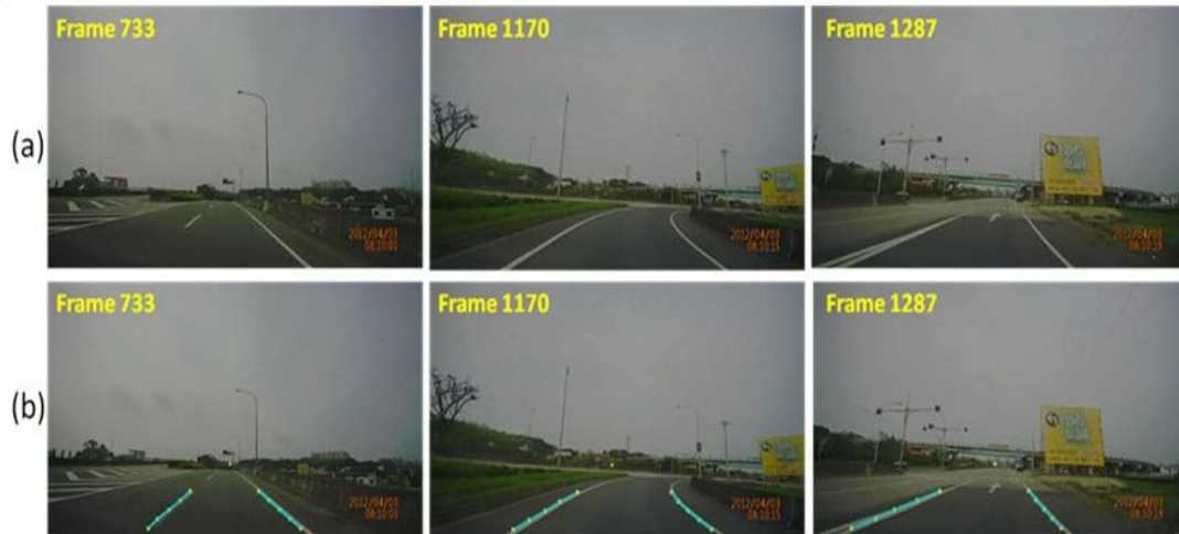
Figure 4-6 : The intermediate case of driving from straight lane lines to curve lane lines then back to straight lane lines. (a) Original images. (b) Output images.
