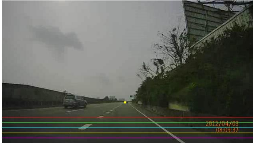
Figure 3-12 : Illustration of ROI setting. The yellow point indicates the final vanishing point, and the five rows ( N_{row} = 5 ) in red, green, cyan, yellow, and purple are the selected ROIs.
