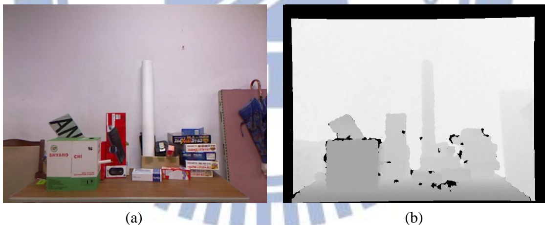
Figure 2.4 (a) the color image captured by CMOS sensor. (b) the depth image captured by Kinect.
