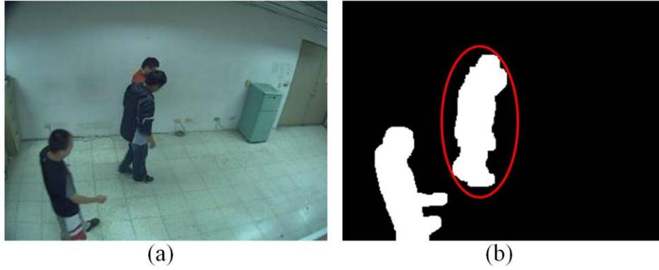
Figure 1.2 An example of serious occlusion in frame 215. (a) The frame shows the person dressed in red jacket is occluded. (b) The binary foreground image of (a).
