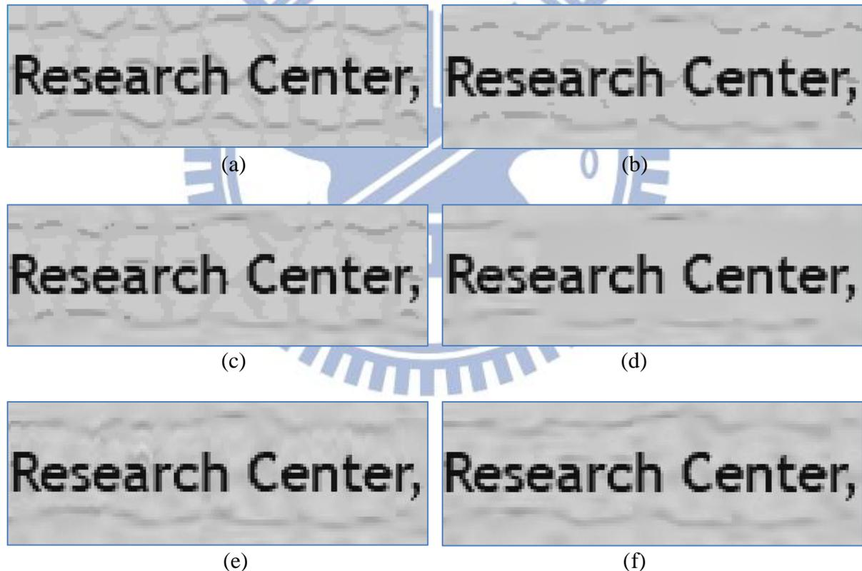
圖 56： *Tile* 在 Qp37 之主觀視覺(a) Original;(b) HM+BCIM: 0.42 bits/pixel;(c) HM+LinearPlane (LC): 0.50 bits/pixel;(d) HM+LinearPlane (GT): 0.39 bits/pixel;(e) HM+SADCT (GT): 0.41 bits/pixel;(f) HM+Matching Pursuit (GT): 0.42 bits/pixel;
