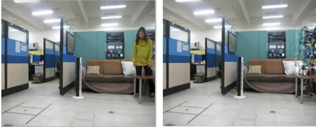
Figure 5.3 Comparison between the original image and the image whose Y2 coefficients have been lost. (Left) the original image. (Right) the image whose Y2 coefficients have been lost.
