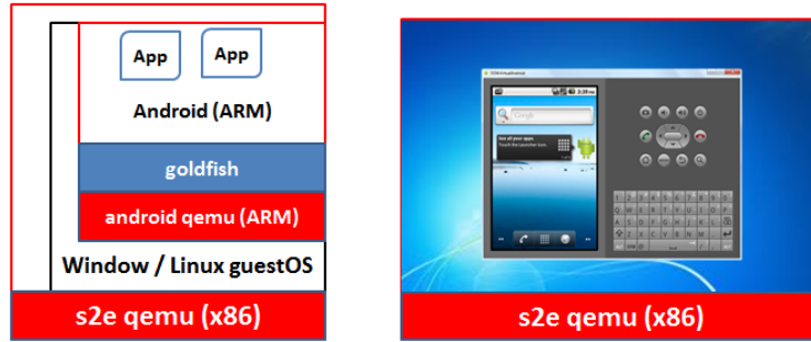
Figure 10: The architecture of ARM Android on top of S 2 E and the screenshot of the Android emulator that emulates virtual smartphone devices to run Android software stack on x86 S 2 E QEMU.
