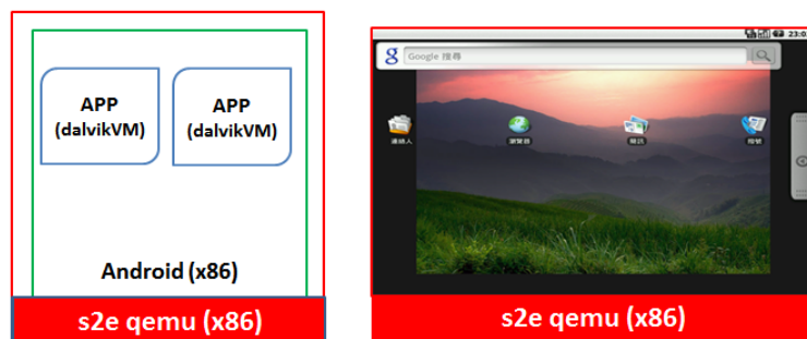
Figure 11: The architecture of x86 Android on top of S 2 E and the screenshot of the x86 Android run as native operating system.
