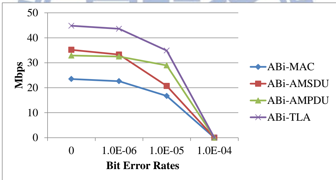
Figure 6.7 Maximum Application Layer UDP Throughput of ABi -MAC with different Bit Error Rates (with UDP payload 1450 bytes, TXOP_{CR} = 10 )
