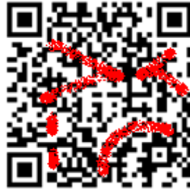
Figure 2-4 Damaged QR Code
