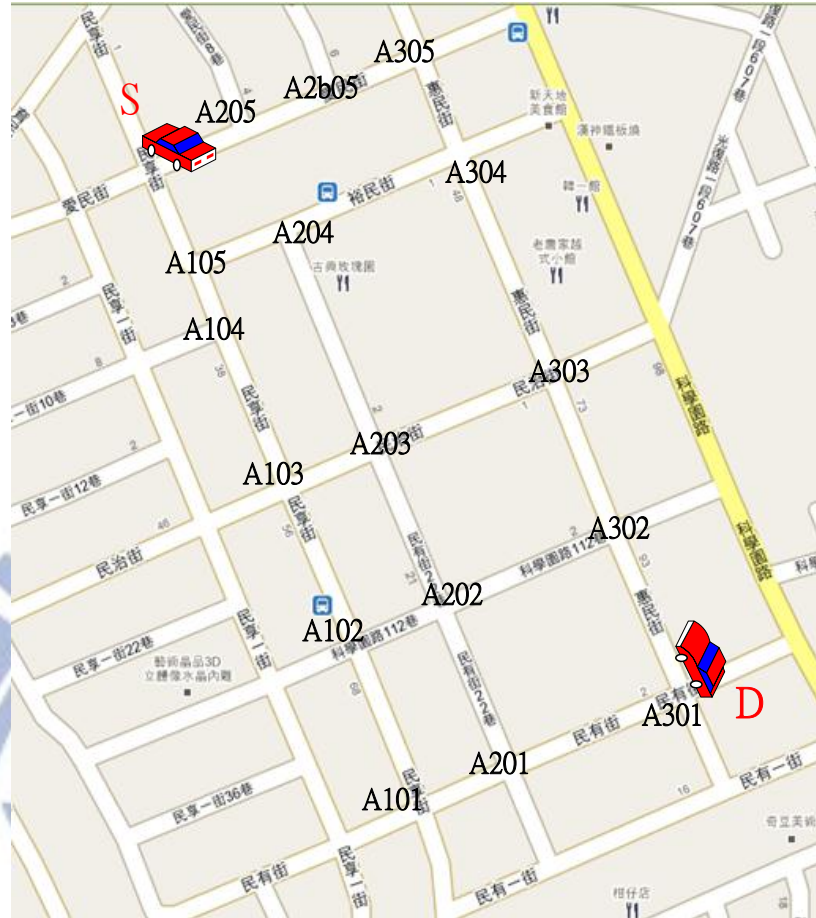
Figure 2. An example of specifying virtual cell IDs on road intersections.
