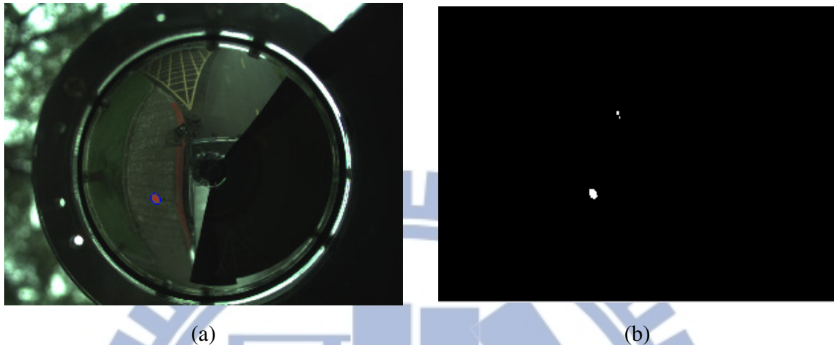
Figure 7.4 An experimental result of landmark detection. (a) An elliptical-shaped landmark in the omni-image. (b) Image of landmark detection by region growing.
