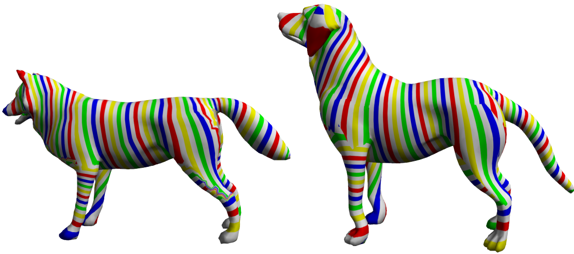
Figure 4.11: Using colored ribbon to show the inter-surface mapping from Wolf to Dog.
