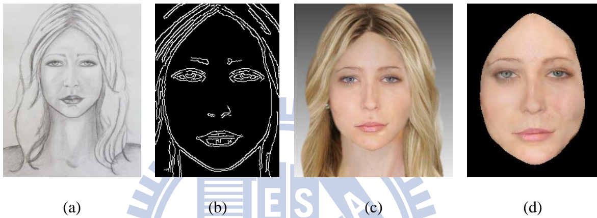
Figure 5.5 (a) The input sketch painting (b) The edge from Canny edge detector (c) Result with edge penalty term (d) Without edge penalty term
