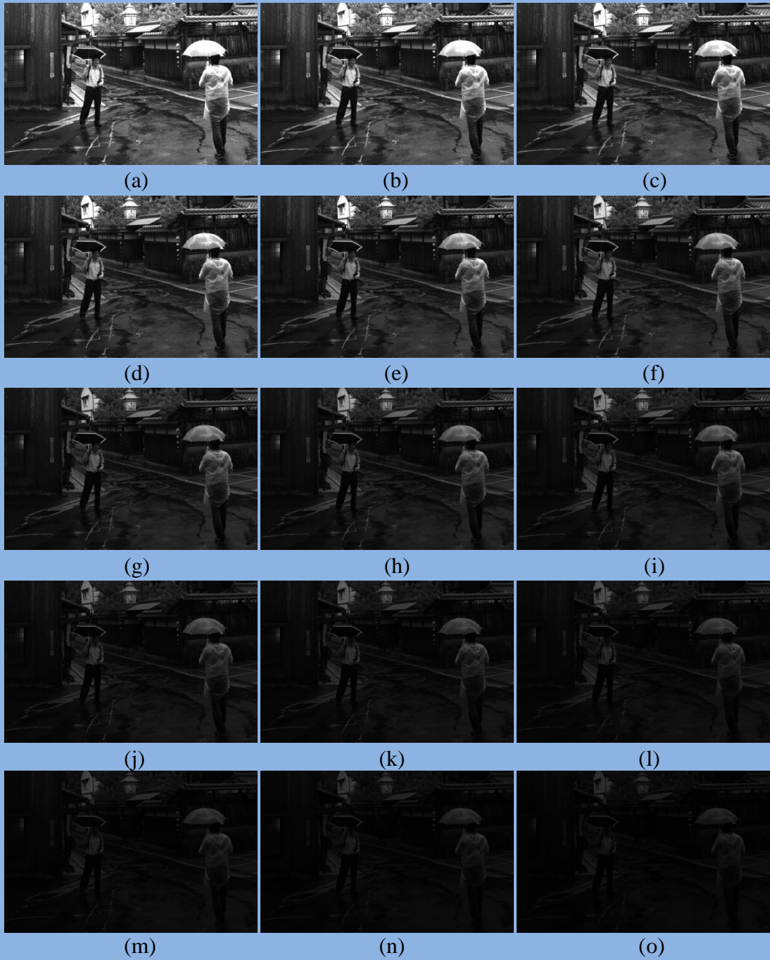
Fig. 3 Generated virtual exposure images (a) k = -7 (b) k = -6 (c) k = -5 (d) k = -4 (e) k = -3 (f) k = -2 (g) k = -1 (h) k = 0 (original image) (i) k = 1 (j) k = 2 (k) k = 3 (l) k = 4 (m) k = 5 (n) k = 6 (o) k = 7
