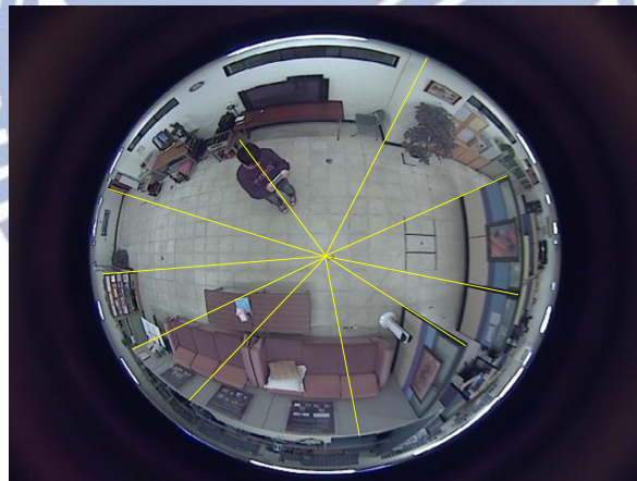
Figure 4.2 Extended image lines of space lines which are perpendicular to the ground will pass through the image center.
