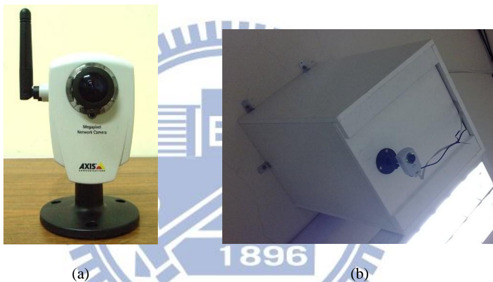
Figure 2.2 The camera used in the proposed system. (a) The appearance of the camera. (b) The camera installed on the ceiling in the indoor environment.
