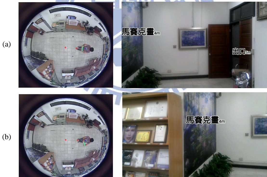
Figure 7.2 A result of browsing visiting targets at a certain location. The left-hand side is the images captured from the fisheye cameras, and the right-hand side is the augmented images shown on the user's mobile device.
