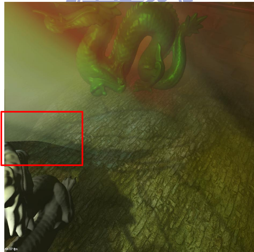
Figure 5.3 Artifacts when reused frame number exceeds a number. (a) Normal (b) with artifacts
