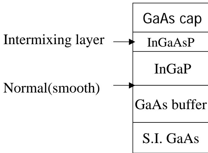
Fig 1.3a The diagram of the GaAs/InGaP/GaAs heterostructure with an inserted InGaAsP layer.
