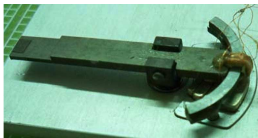
Fig. 17. Fabricated seesaw swing arm VCM actuator.
