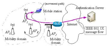
Fig. 1. Under IEEE 802.11r the first (re)association in a mobility domain requires IEEE 802.1X authentication. The established security context will be distributed from the first reassociated AP to other APs along with the MS's movement in the same domain whenever necessary.
