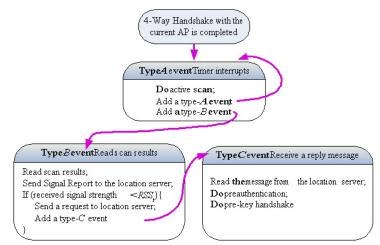
Fig. 7. A diagram of event handling at mobile client sides. The handling process involves three types of events.
