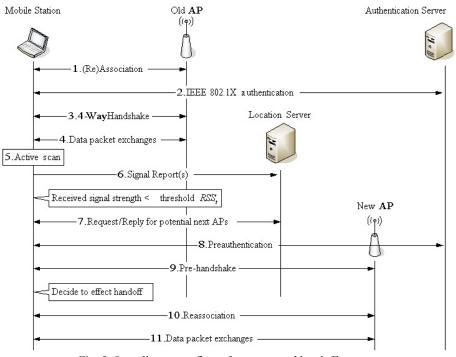
Fig. 5. Overall message flow of our proposed handoff process.
