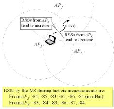
Fig. 4. Changes of RSSs by an MS with respective APs suggest to which APs the MS tends to reassociate next.
