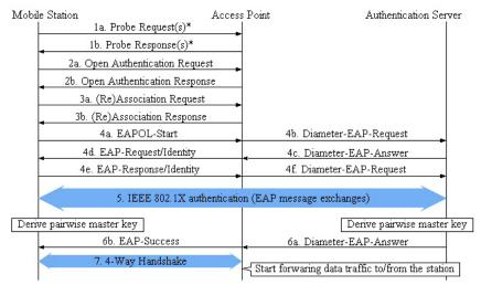
Fig. 2. Message flow for an MS handed off to an AP in standard IEEE 802.11i settings. Message marked with '\*' may be not present.
