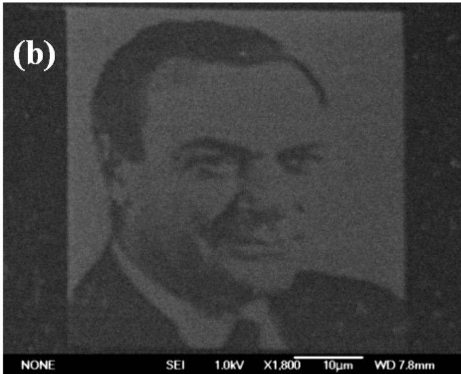
Figure 4.16 (a) Black and white gray-level photograph of the physicist Richard P. Feynman (Resolution: 512 \times 512 ); (b) SEM images of the AuNPs selective gray-level patterning on the \text{SiO}_2 surface by applied the low energies of additional bias after immersion in the AuNPs solution for 1 h. (SPL gray-level patterning voltages from 2.5 V to 5.5 V, the resolution of SPL bond breaking patterning is 11.71875 mV/grad, and the pitch of pixel is about 97.66 nm).
