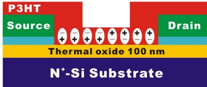
Figure 7-8 Directions of dipoles in the organic active layer when V_G = -10 V, V_D = -20 V and V_S = 0 V
