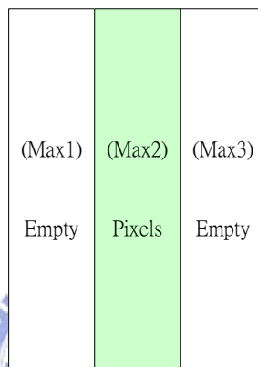
Figure 4.2 The max bin is quantized into three parts.
