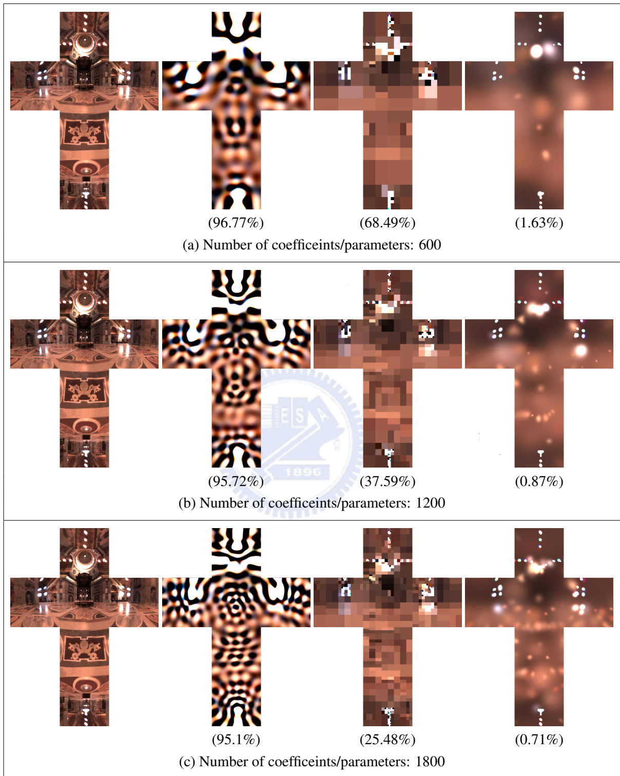
Figure 7.3: Reconstructed images of the HDR environment map St. Peter's Basilica based on different functional representations. From left to right in each row: raw data; spherical harmonics; area-weighted Haar wavelets [125]; scattered univariate SRBFs with non-negative basis coefficients. The squared error ratio of each reconstructed image is shown in parentheses.
