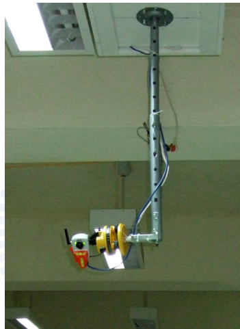
Fig. 6.11 Fish-eye camera used in this study, which is attached to a rod fixed on ceiling and can be tilted and moved up and down.
