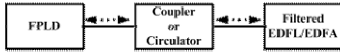
Fig. 2.2 The mutually injection seeding scheme between FPLD and filtered EDFL (or EDFA).
