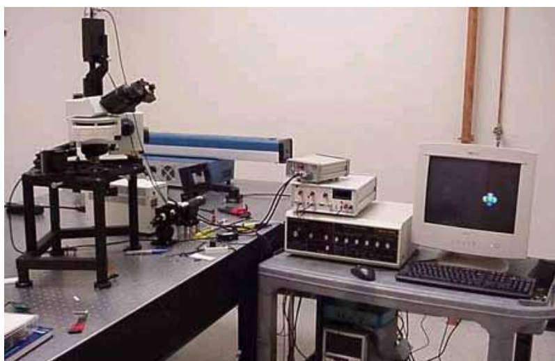
Fig. 5-6 The schematic diagram of NSOM
