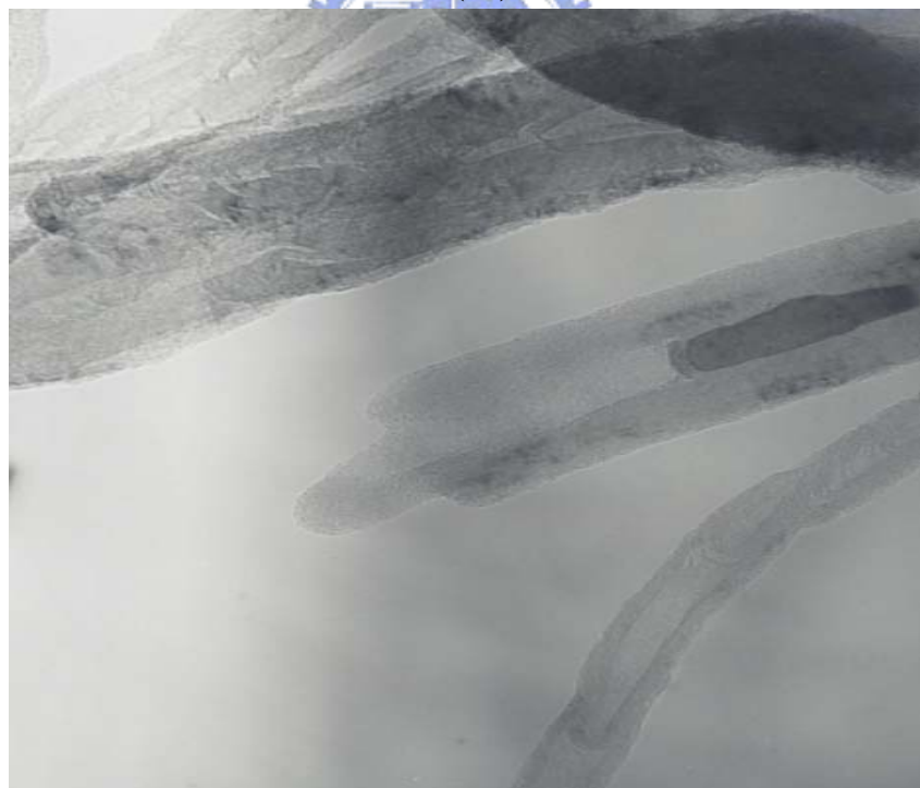
Figure 6-6 TEM images of CNTs (a) before and (b) after O_2 plasma post-treatment. The plasma power and treatment time were 400 W and 60 s, respectively.
