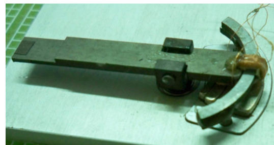
Fig. 5. (Color online) Fabricated “seesaw-shaped” VCM actuator.
