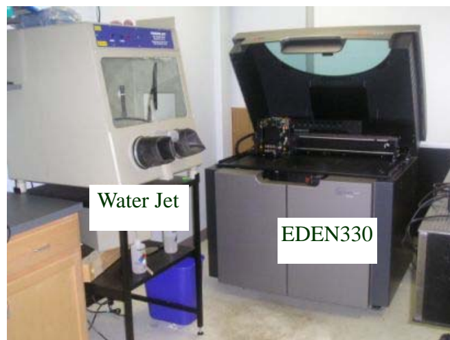
Fig. 2.9 The EDEN330 Rapid Prototyping device and water jet.
