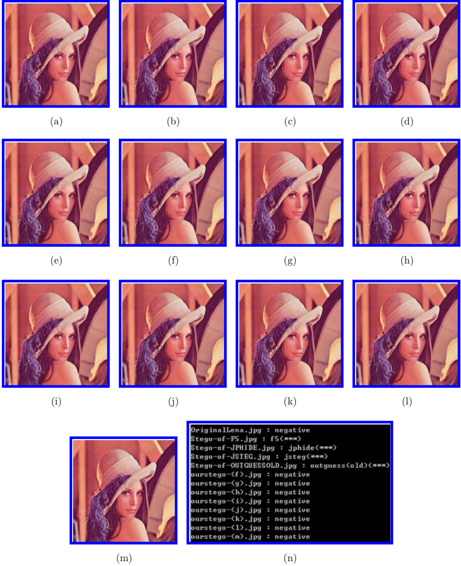
Fig. 7. Results of Stegdetect analysis: (a) the image decompressed from the JPEG-Q85 code without any hidden secret; (b)–(e) the stego-images decompressed from the JPEG stego-codes for F5, 25 JPHide, 13 Jsteg, 22 OutGuess, 17 respectively. (f)–(m) the stego-images decompressed from our eight JPEG stego-codes, respectively; (n) the results of Stegdetect analysis of the thirteen JPEG codes, the decompressed images of which are in (a)–(m).
