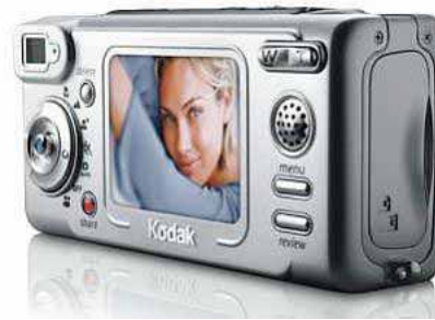
Figure 1-1 The first full color AMOLED product of DSC demonstrated by Kodak-Sanyo in 2004.
