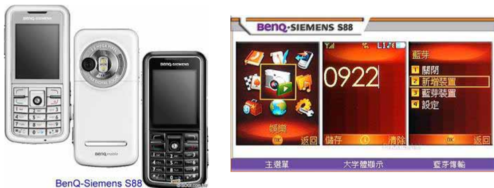
Figure 1-3 The first full color AMOLED product of mobile phone demonstrated by BenQ-Siemens (AUO) in 2006.
