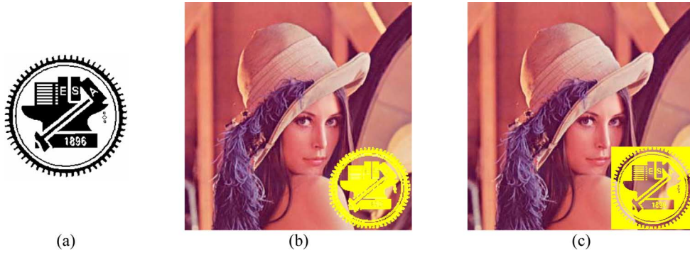
Fig. 2. Illustration of pixels in a watermark. (a) A monochrome watermark. (b) Area of P (yellow pixels). (c) Area of P' (yellow pixels).
