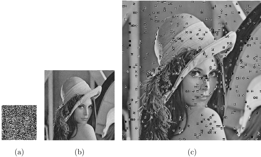
Figure 4.7: A received and reconstructed image from an erroneous channel. (a) The extracted 128 \times 128 watermark. (b) The received watermarked base layer which contains transmission errors. (c) The reconstructed 1024 \times 1024 image.
