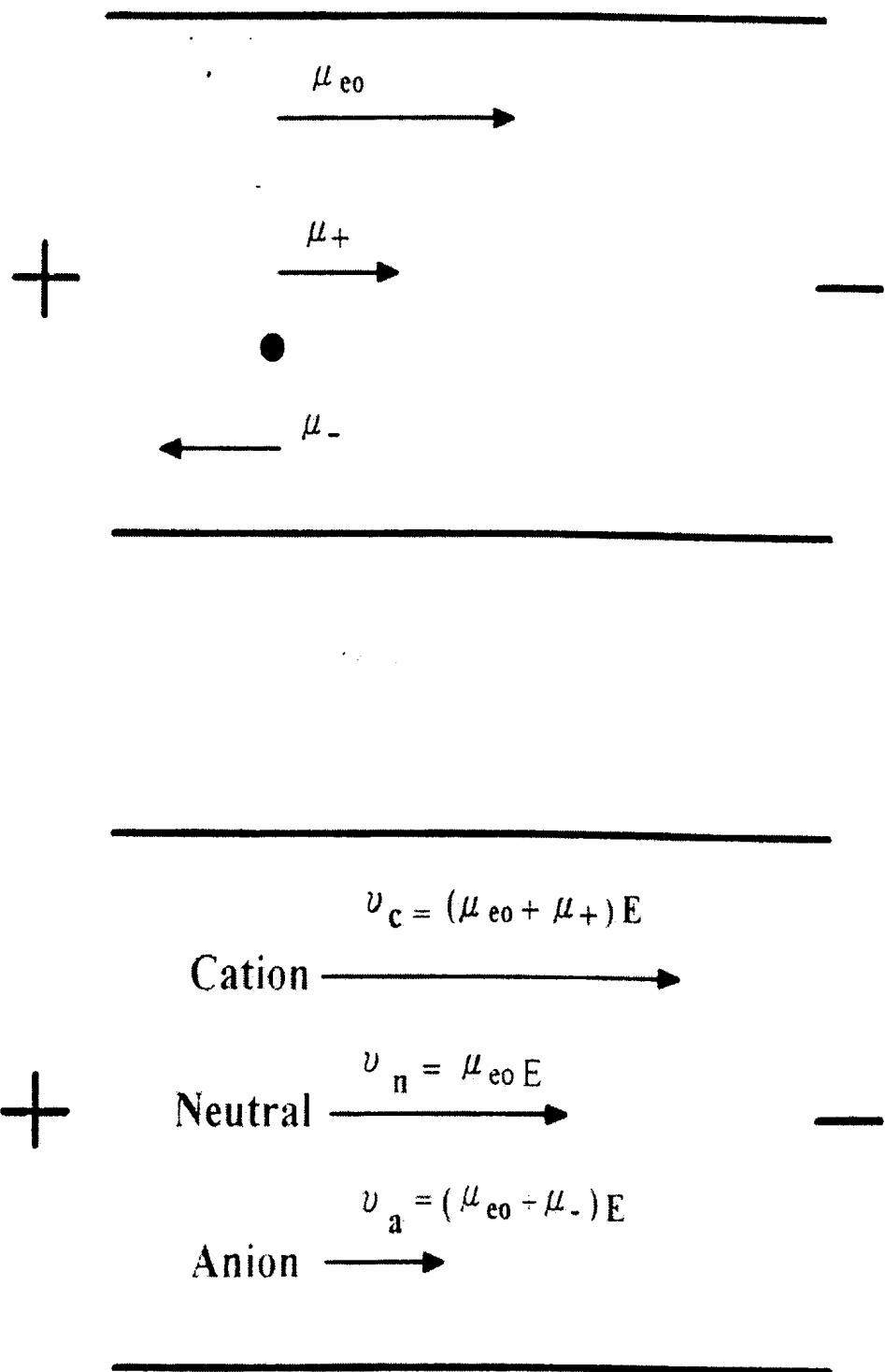
Fig. 2. Electrophoretic mobility of analyte
