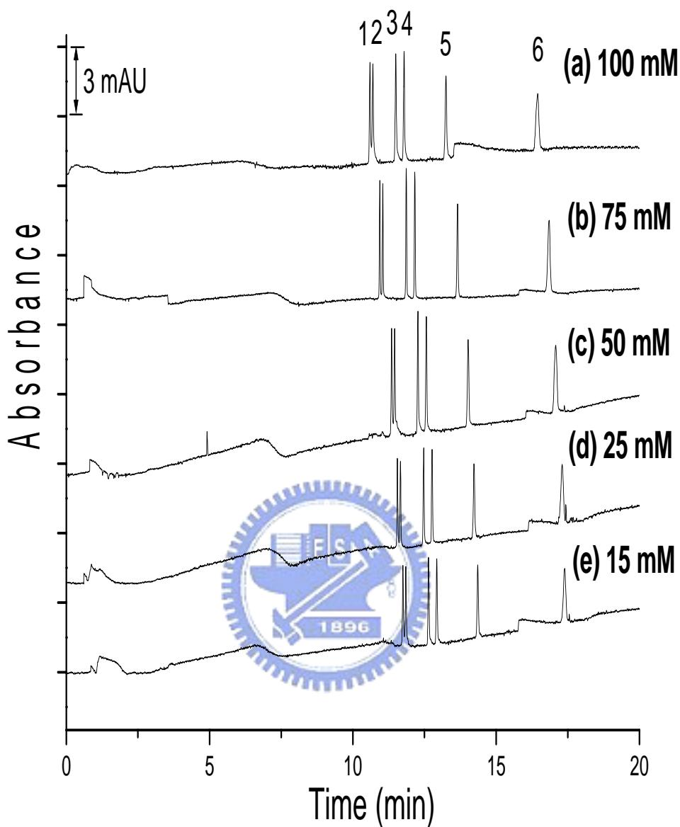
Fig. 19. Effect of the concentration of sample matrix.
