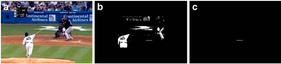
Fig. 5 Procedure of home plate detection. a Original frame of a pitch scene, b pixels with high intensity around the frame center, c detected home plate
