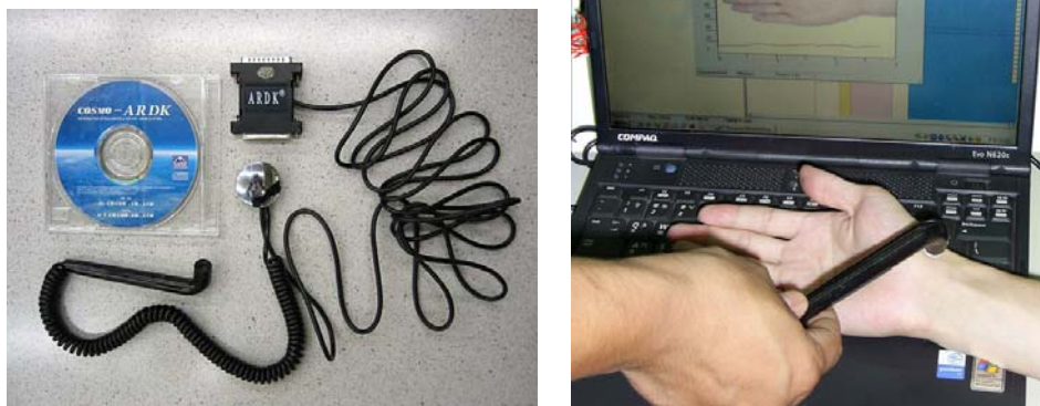
Fig. 2-1 The measurement probe (left) and the measurement window (right) of ARDK
