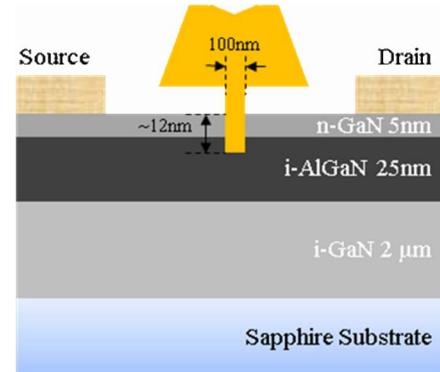
Fig. 1. Cross section of the 100-nm-gate-recessed n-GaN/AlGaN/GaN HEMT.
