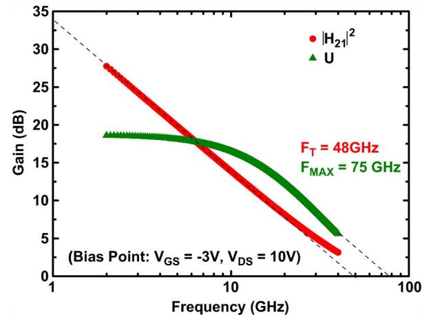
Fig. 3. Intrinsic  $S$ -parameter performance of the device at the bias point of  $V_{GS} = -3 \text{ V}$  and  $V_{DS} = 10 \text{ V}$ .
