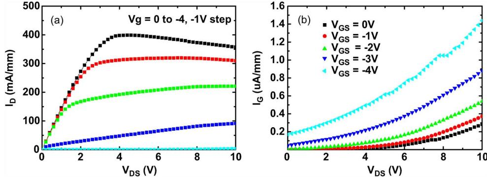
Fig. 2. (a) DC forward characteristics of the 100-nm-gate-recessed n-GaN/AlGaN/GaN HEMT. The source-drain spacing and device size are  $7 \mu\text{m}$  and  $2 \times 50 \mu\text{m}$ , respectively. (b) Gate leakage current density during the device operation.
