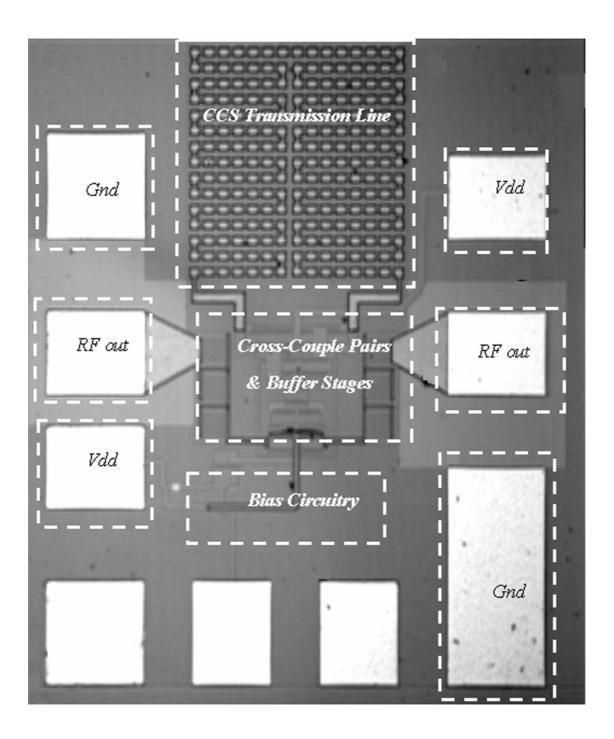
Fig. 4.7. 5.2-GHz CMOS cross-coupled oscillator based on a CCS TL resonator. Chip area: 0.5 mm  $\times$  0.6 mm (including pads), 0.225 mm  $\times$  0.21 mm (active area), and 0.225 mm  $\times$  0.225 mm (CCS TL on top).
