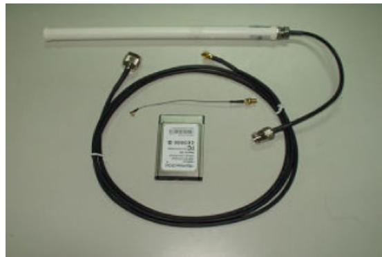
Fig. 14. The external antenna, cable, and wireless NICs used in field trial.
