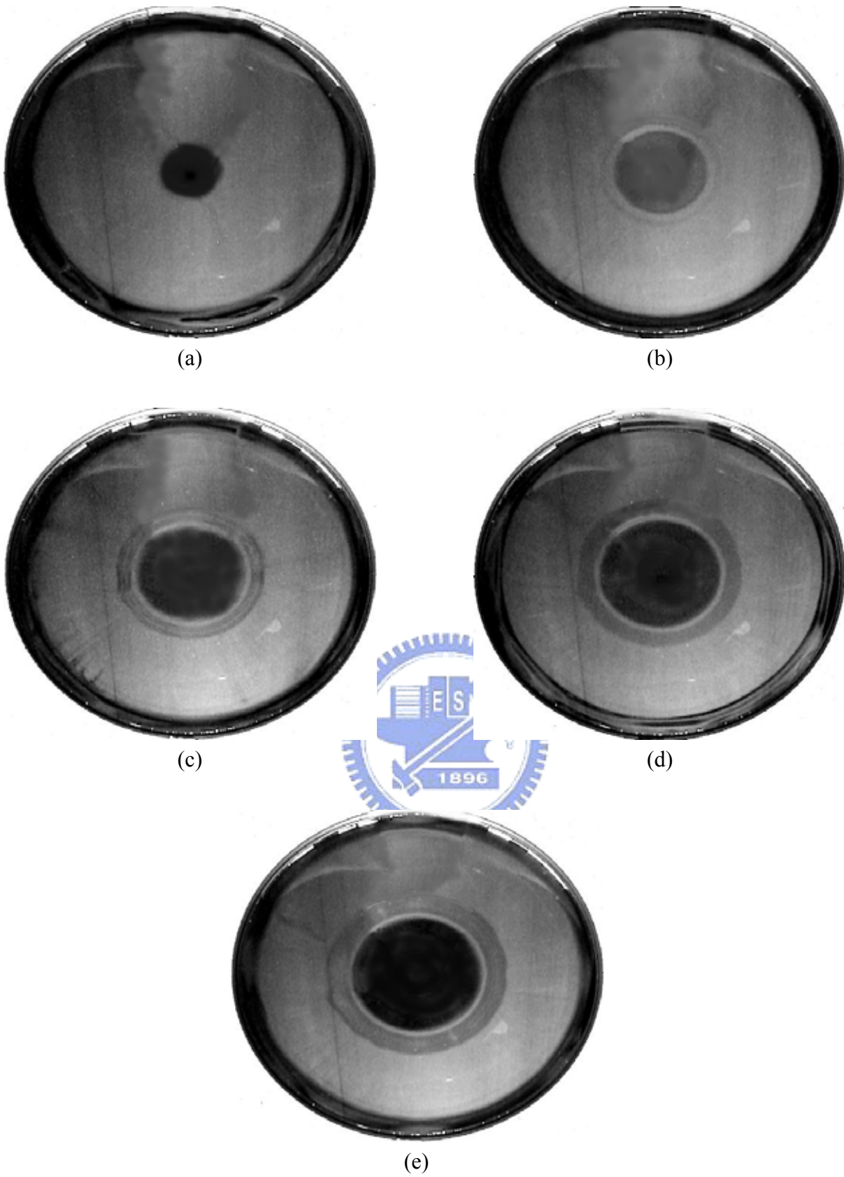
Fig. 3.18 Steady top view flow photos taken at the middle horizontal plane between the disk and chamber top with Ra=0 ( \Delta T=0^\circ\text{C} ) & D_j=10.0 mm at H=15.0 mm for Re_j= (a) 135, (b) 270, (c) 406, (d) 541, and (e) 676.
