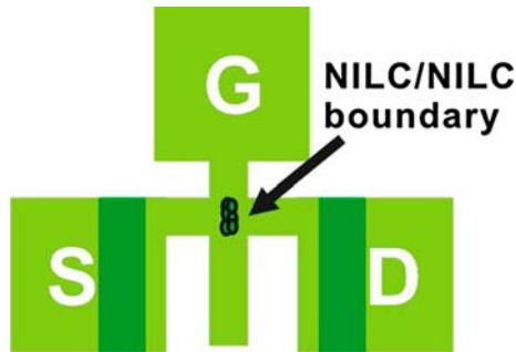
Fig. 1. Schematic illustration of the TFT device.
