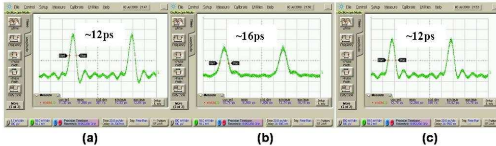
Fig. 5. The measured optical pulse by using 50 GHz photodiode (a) without fiber link, (b) 250 m SSMF, and (c) 250 m SSMF and 50 m DCF.
