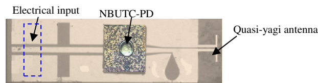
Fig. 2. Photograph of the novel W-band NBUTC-PD used for the UWB-IR system.
