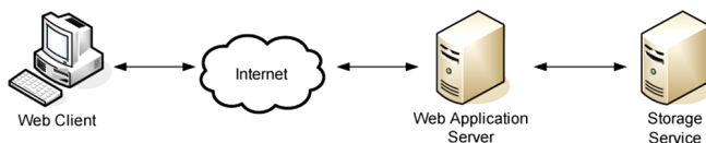
Figure 1 The architecture of a typical web system with external storage service (see online version for colours)
