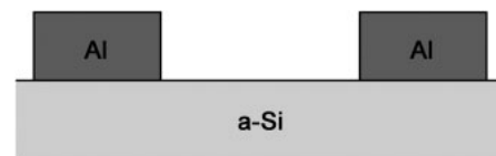
Fig. 1. Illustration of the cross-sectional structure of the sample after removing the photoresist patterns.
