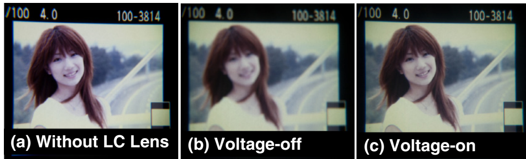
Fig. 4. (Color online) (a) Image obtained from the manually focusing pico-projector without the LC lens. d = 0.625 mm and s' = 50 cm. (b) Images obtained from electrically tunable focusing pico-projector at (b) V_o = V_H = 0 and (c) V_o = 43 V rms and V_H = 90 V rms . d = 0 and s' = 50 cm.
