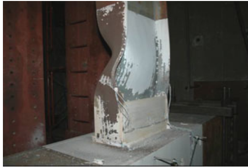
Figure 7. Specimen SP1 beam buckling (4.7% drift).
