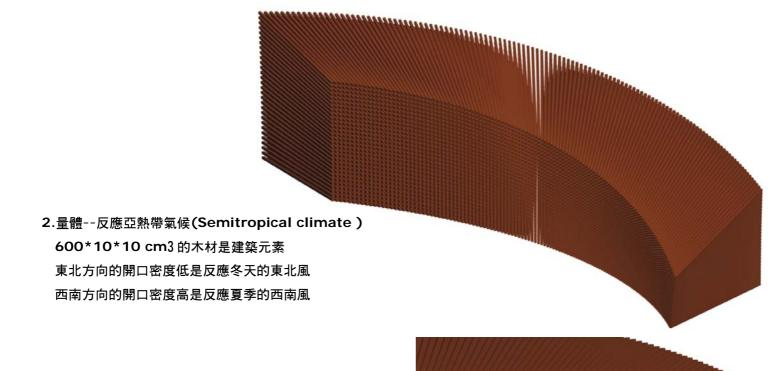
2. Object ---Reflect Semitropical Climate 600 cm by 10 cm by 10 cm timber construct the main element of the ecohouse. In order to reflect winter monsoon, the density of the building opening toward the northeast face is lower; on the other hand, the southwest face is higher to reflect the summer monsoon.
